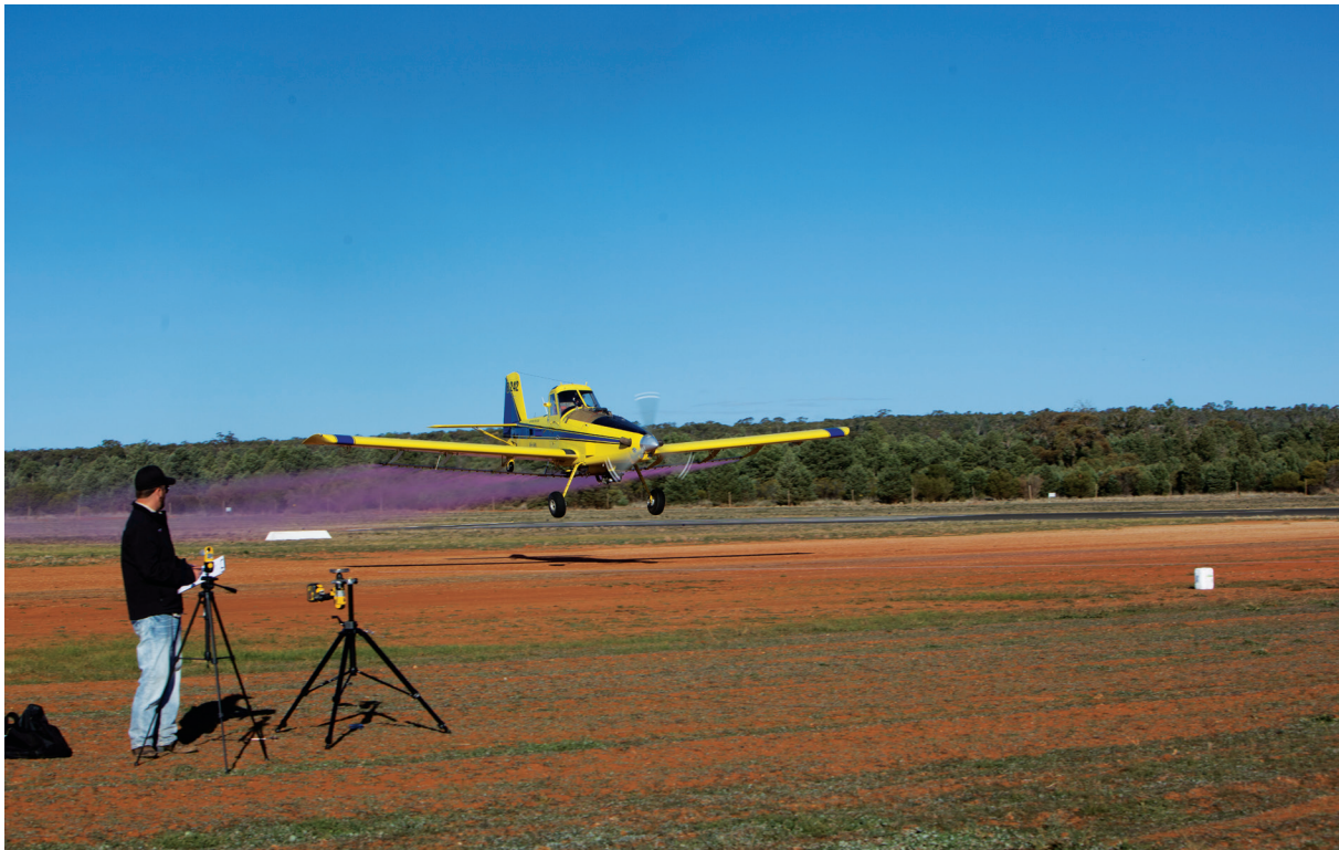
Figure 7.6: Aircraft set-up makes a big difference which is why pattern testing is used extensively (Photo: Adam Hooper)
